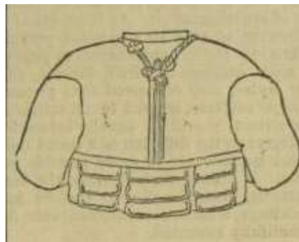
Figure 19: John Dennis Caulcher's design for a cork lifejacket.
