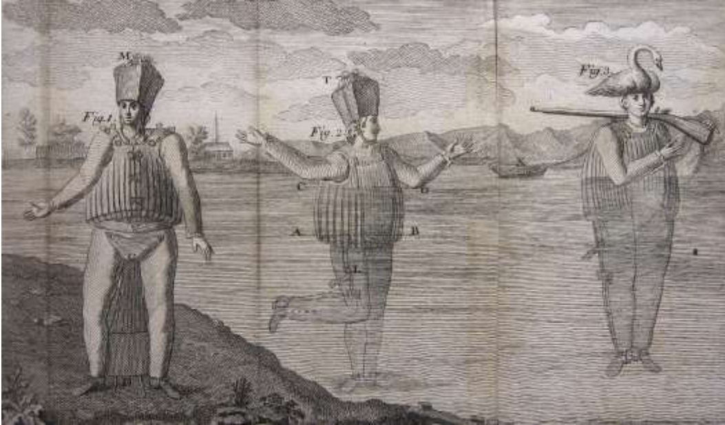
Figure 10: Jean-Baptiste de la Chapelle's design for a "flotation suit" made with cork.
